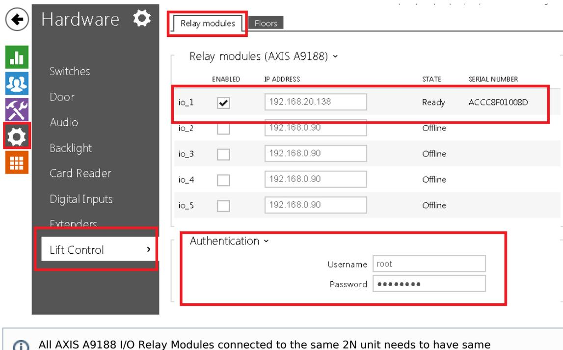
administrator user with same password (root for example) - maximum of 5 AXIS A9188 I/O Relay Modules can be connected to one 2N unit allowing for maximum of 40 floors
