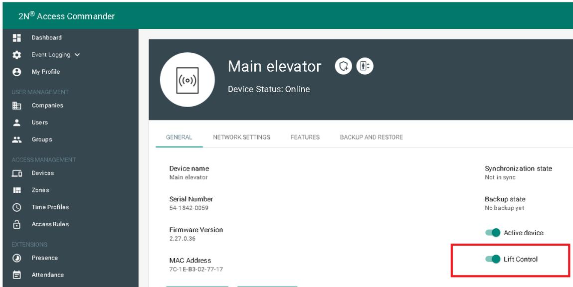
**i** If you add to Access Commander device with lift control license, it will become automatically enabled for Lift Control)
